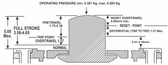
The repeat accuracy of individual switch trip points is such that after millions of operations they do not drift more than two or three thousands of an inch.
