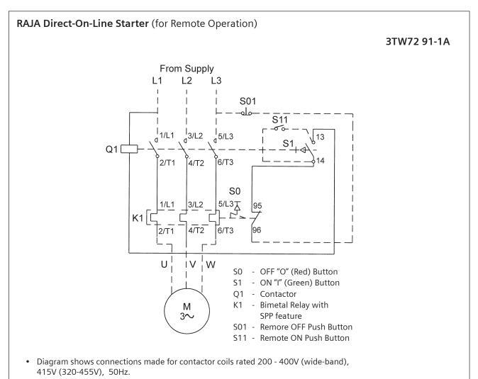
• For remote operation disconnect the wire between terminal 5/L3 on contactor and terminal 96 on the relay. Connect the remote 'OFF' S01 push button as shown. Connect remote 'ON' S11 push button parallel to S1 as shown.
