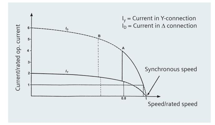
In star delta starting, initially the motor windings are connected in star. This reduces the starting current by 1/3 rd of the full load current also the voltage by  $(1/\sqrt{3})$  of the rated value. As the torque is proportional to the square of the voltage, the starting torque also get reduced to 1/3rd of it's full load value. Once the motor attains approximately 80% of the rated speed, the windings get connected in the delta formation.
