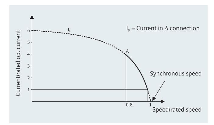
The most economical and popular method of starting squirrel cage induction motors, is direct-online, where the starter is connected directly across the supply. However, the starting current at the moment of switching Direct-on-line can be as high as 6-8 times the rated current.
