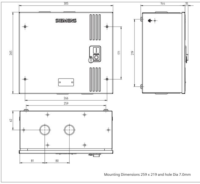
Fig. 8: Dimensional Details for 3TE72 91-0A\*\*
