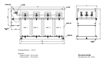
${\bf Drawing\,10\,\text{--}Three\,Phase, Rectangular\,Capacitor}$
