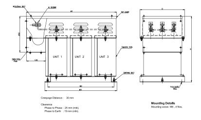
Drawing 5 - Three Phase, Rectangular Capacitor Bank (Four Unit)
