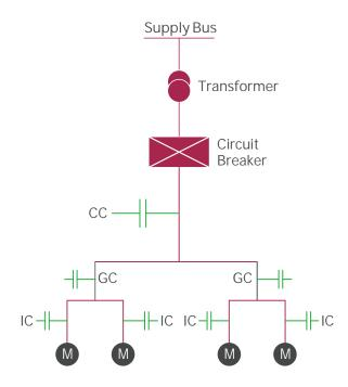
CC=Central Compensation GC=Group Compensation IC = Individual Compensation M = Motor Load
